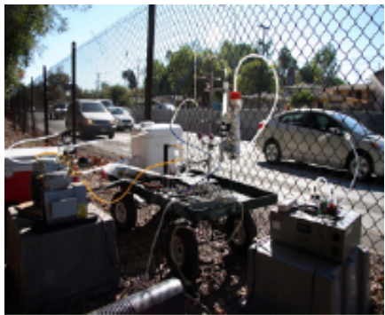
Emissions testing station located near the 110 freeway.
